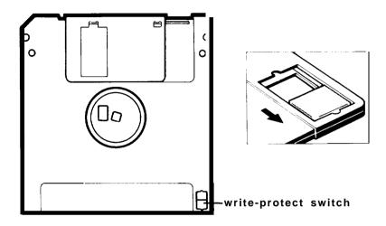
To remove the write protection, slide the switch toward the center of the diskette until it clicks into position and the hole is covered.
